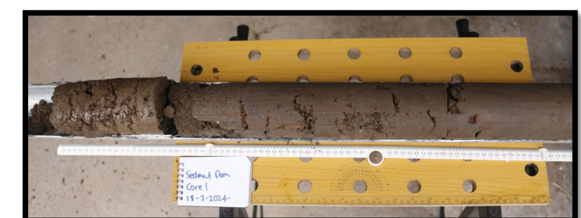
Fig 5. A soil core from the sediment pond. Soil cores indicated a sediment depth of 120 cm.
