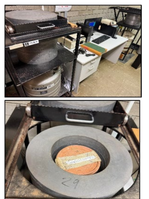
Fig 3. Hyperpure germanium detector used ^{137}\text{Cs} analysis.
