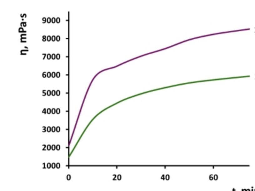
Comparison of the cross-linking kinetics of the **SA/HA 75/25** system without inhibitor (1) and with inhibitor (2)
