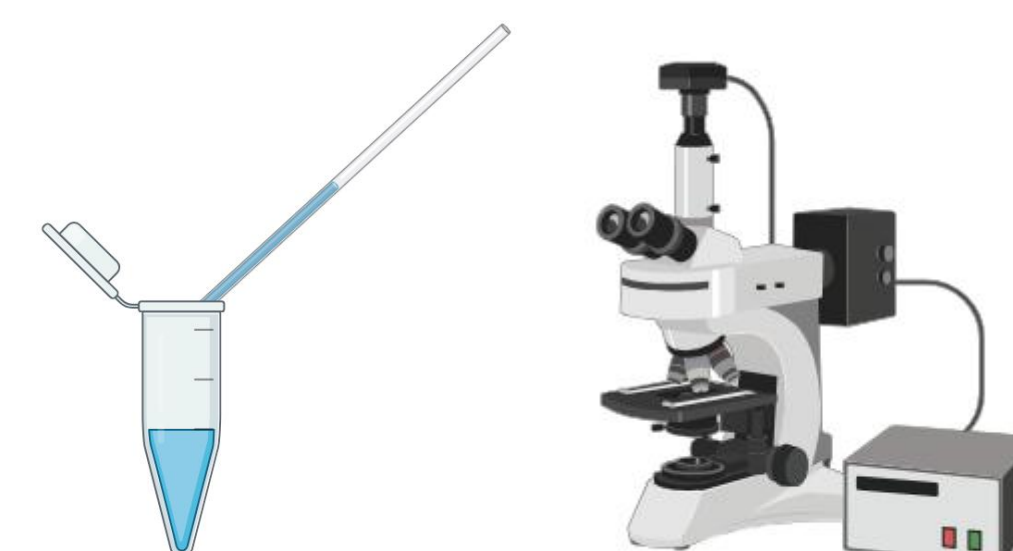
Figure 2. Deposition of phage in capillary tubes and examination under polarized optical microscopy (POM). Created in Biorender.com
