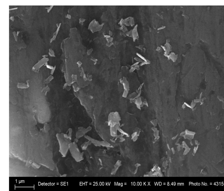
Fig. 4. SEM image of exfoliated PdSe 2 crystal
