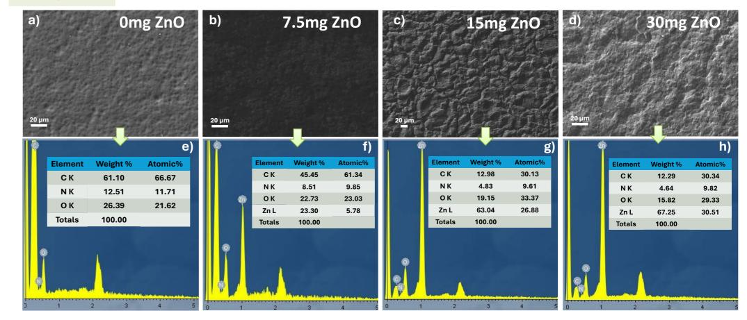
From Elemental mapping (EDS) of Zn in Pol/ZnO membranes it is seen that: there is good distribution of ZnO in the hybrid membranes, and the signal of Zn is increased with increasing ZnO in composition.
