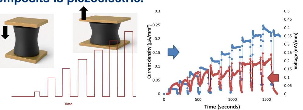
The maximum power density extracted under periodic strain and matched load conditions reached  $\sim$ 7 nW/cm³ at 1 k $\Omega$  [1].
