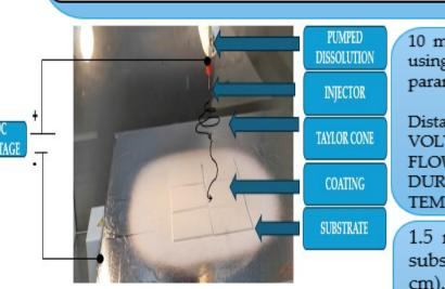
Electrospinning setup for the PLA+Lignine membranes over glass substrates (72x52 mm)
