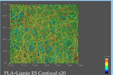
The diameters of the PLA electrospun fibers was 2.241  $\pm$  1.329  $\mu m$  and for PLA+Lignin 1.639  $\pm$  0.754  $\mu m$ .
