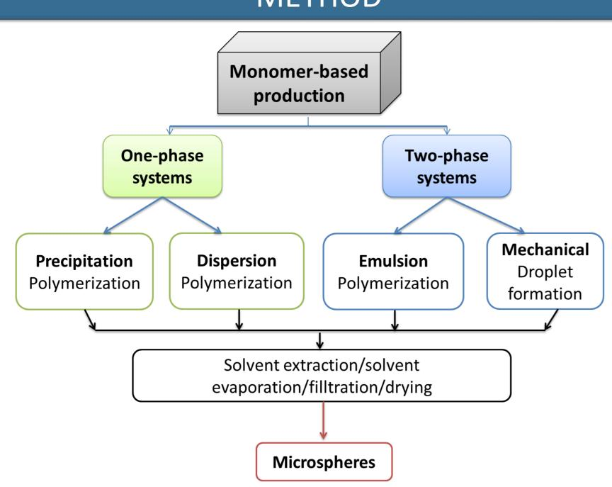
✓ Polymeric microspheres were obtained by polymerization of a water-in-oil (w/o) Pickering emulsion.
