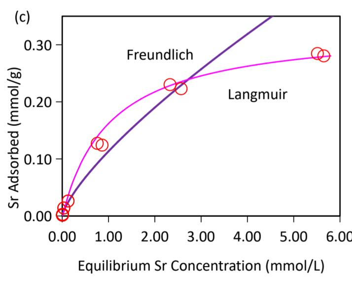
Fig. 1a-b: Sr<sup>2+</sup> sorption kinetics (0.1/10 mM) on Taiwan Zhi-Shin bentonite, pseudo-second-order fit (solid lines) with linear insets. 1c: Langmuir/Freudlich isotherms. 1d: Cation desorption vs Sr<sup>2+</sup> adsorption. 1e: Temperature-dependent adsorption (0.1/10 mM-Sr) with thermodynamics.
