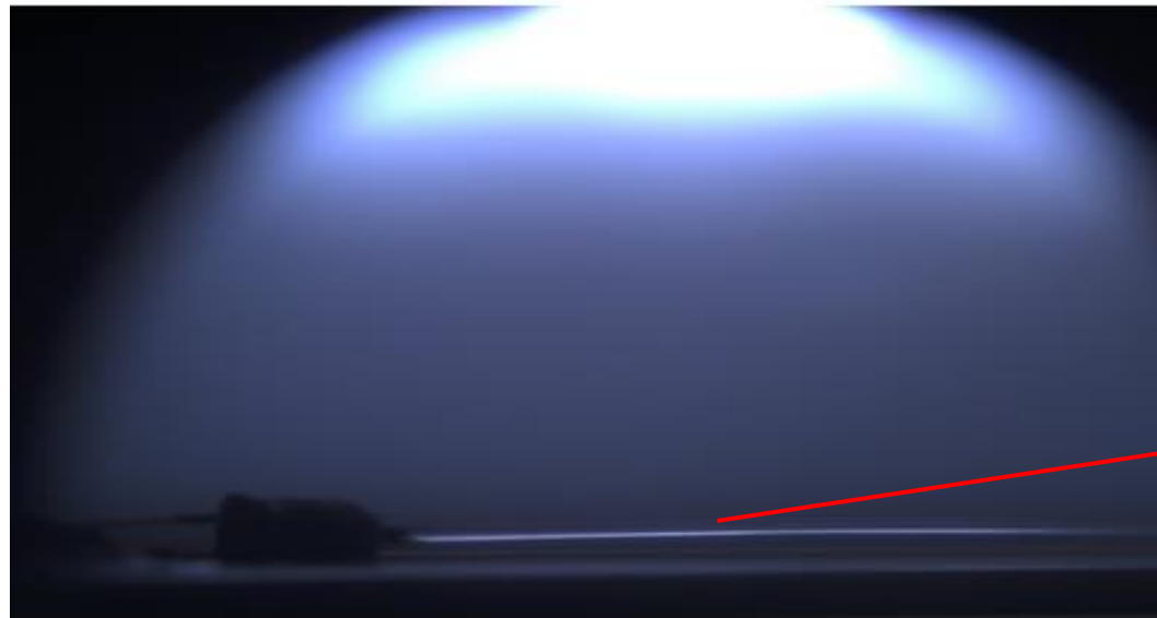
Fiber inside PECVD reactor
