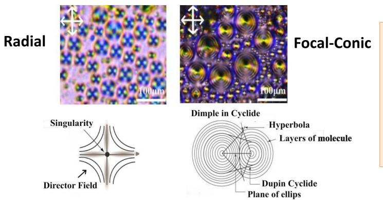
POM observations of 8CB interacting with the HI (20-300 µM, time-dependent) showed two main textures: Radial and Focal conic.
