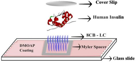
**DMOAP**: dimethyl octadecyl [3-(trimethoxy silyl) propyl] ammonium chloride – Helps in **homeotropic arrangement of LC**
