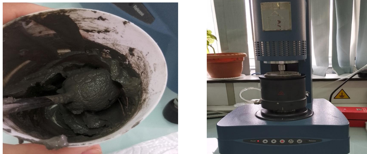
Fig. 4: Cementitious pastes (a) Rheometer AR200- rheological tests (b)
