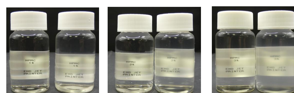
Figure 1. Different HPMC bio-inks concentrations (1, 2 and 3% (w/w) in 80% (v/v) ethanol (left) and 90% (v/v) ethanol (right).
