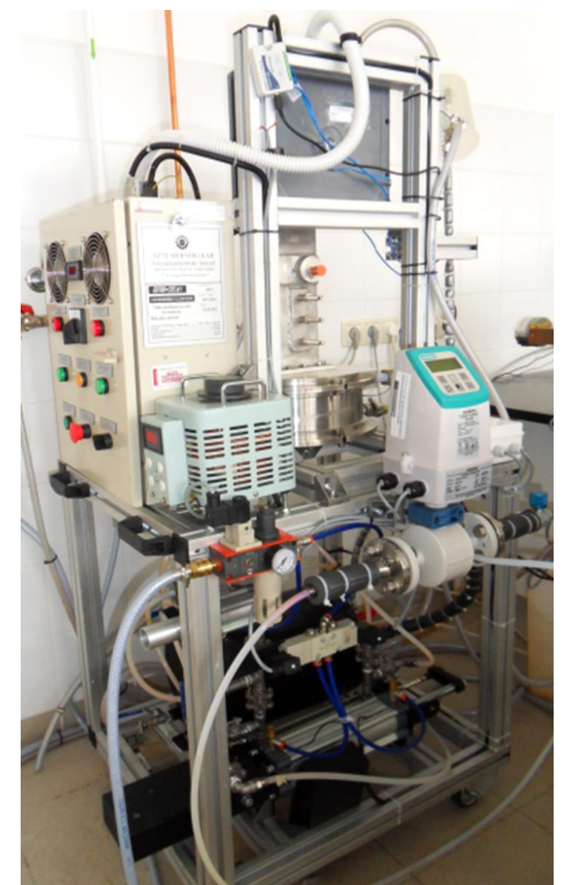
Microwave sludge treatment unit
