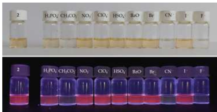
Figure 2. Solutions of compound 2 in DMSO under ( top ) natural light and ( bottom ) UV radiation at \lambda_{\text{max}} = 312 \text{ nm} upon addition of 50 equivalents of various anion solutions.
