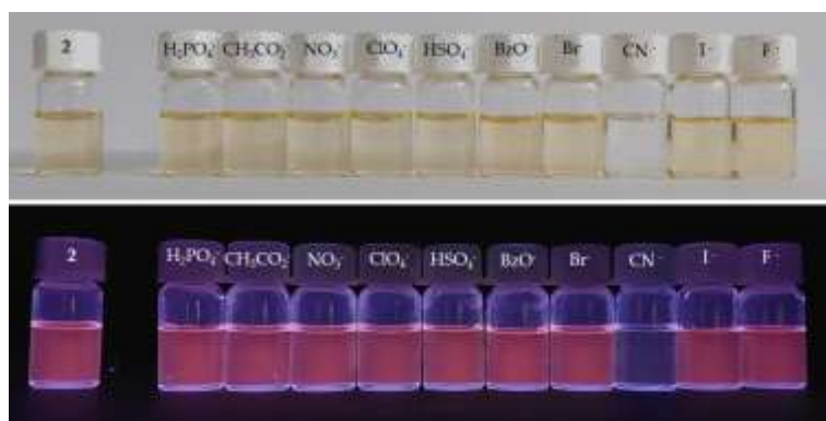
Figure 3. Solutions of compound 2 in DMSO/water (75:25) under ( top ) natural light and ( bottom ) UV radiation at \lambda_{\text{max}} = 312 \text{ nm} upon addition of 50 equivalents of various anions solutions.
