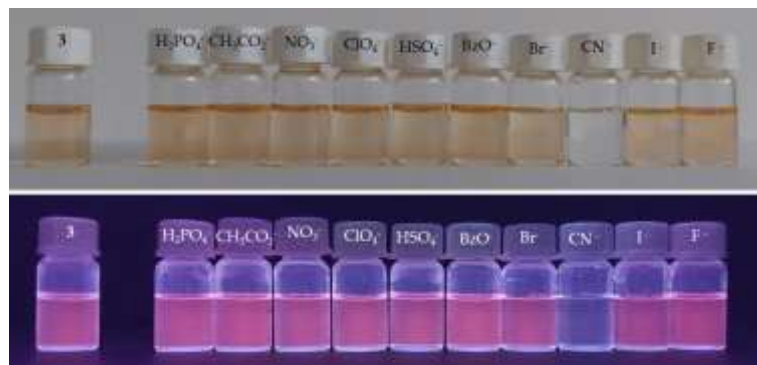
Figure 6. Solutions of compound 3 in DMSO/water (75:25) under (top) natural light and (bottom) UV radiation at \lambda_{\max} = 312 nm upon addition of 50 equivalents of various anions solutions.
