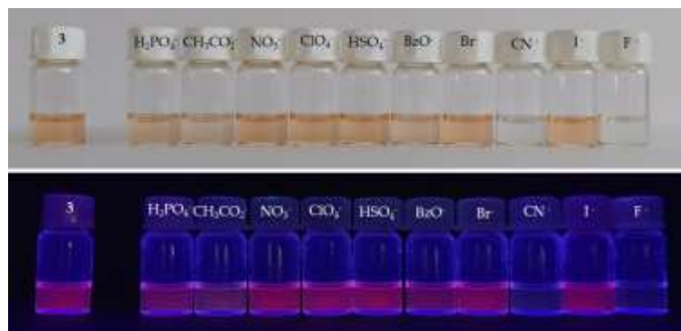
Figure 5. Solutions of compound 3 in DMSO under (top) natural light and (bottom) UV radiation at \lambda_{\text{max}} = 312 \text{ nm} upon addition of 50 equivalents of various anions solutions.
