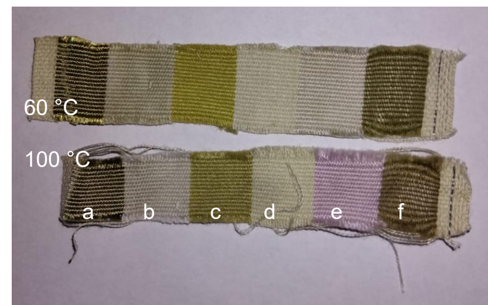
Figure 3: Results obtained from dyeing a multifiber fabric composed by: a) acetate; b) cotton; c) nylon; d) polyester; e) acrylic; f) wool, at both temperatures
