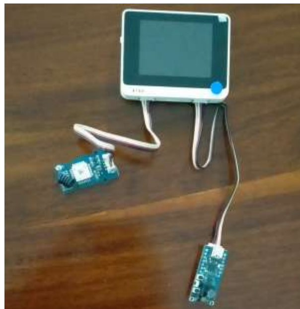
Figure 2. SenseCAP K1101 (Wio Terminal + Vision AI Sensor + LoRa Module).
