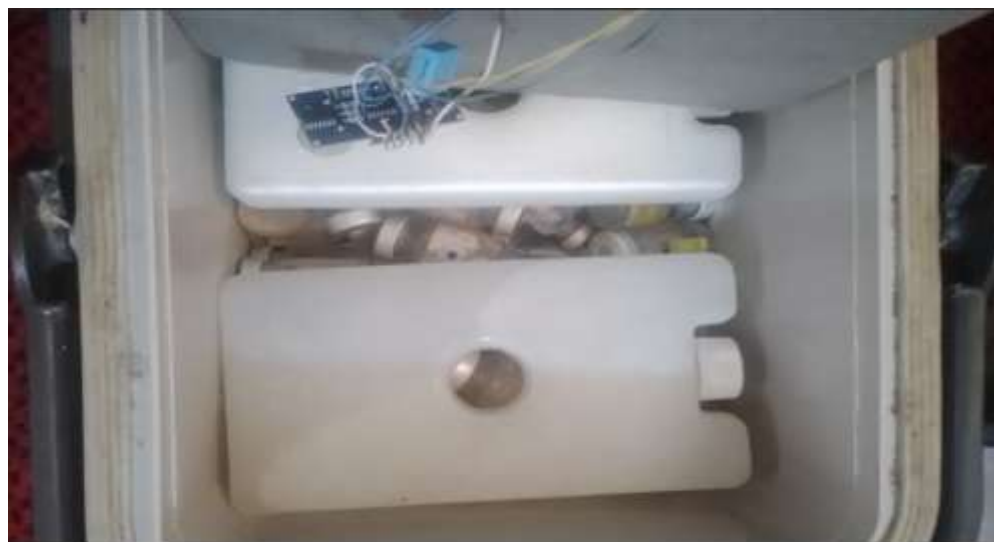
Figure 5. Prototype testing using COVID-19 vaccines in Gio's style vaccine carrier.
