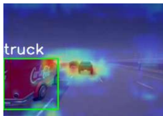
Figure 3. Grad-Cam and Faster RCNN output image applied on camera image.
