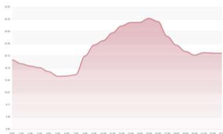
Figure 4. Atmospheric temperature data read from BME280 during bench test.
