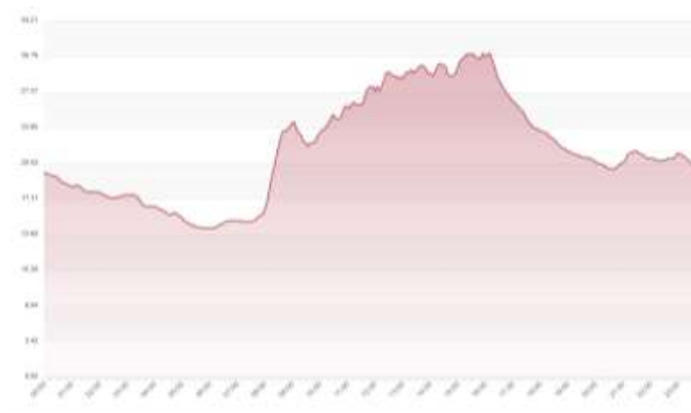
Figure 5. Soil temperature read data from DS18B20 during bench test.
