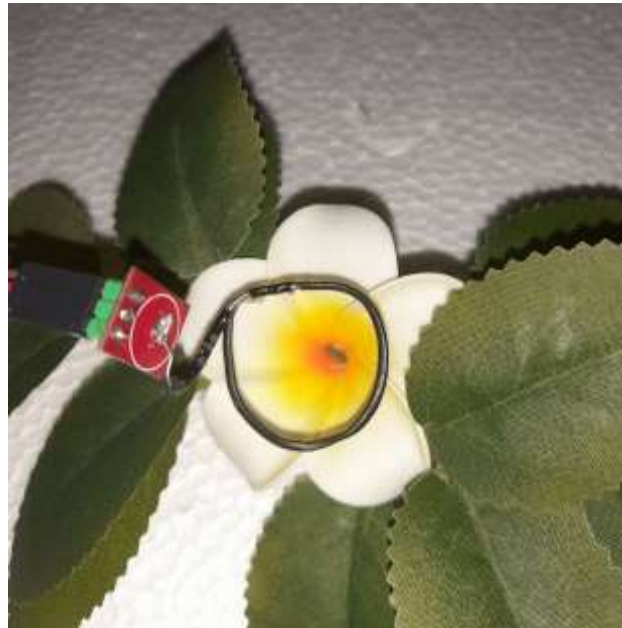
Figure 5. Capacitive touch sensor with additional wire.
