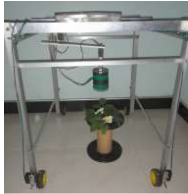
Figure 1. Rover with robotic arm on top of testing flower setup.
