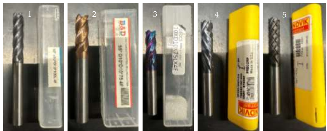
Figure 4. Milling Cutters used (1) Titanium Carbo-Nitride Coating, (2) Naco4 Coating, (3) Nano Blue Coating, (4) Coromill Plura 2P460-AO and (5) Coromill Plura 2P350-AO.
