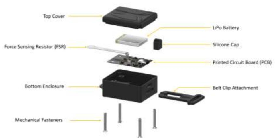
**Figure 1.** Exploded view of the proposed wearable respiratory monitoring device.
