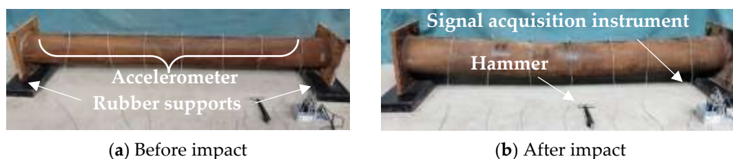
Figure 1. Modal testing setup.
