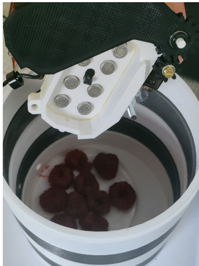
Figure 5. Experimental setup to measure raspberry odor.
