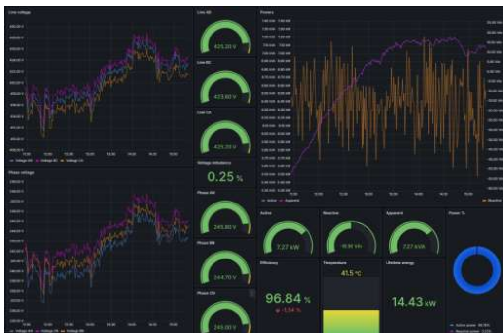
Figure 12. INVERTER dashboard voltages and powers detailed view.
