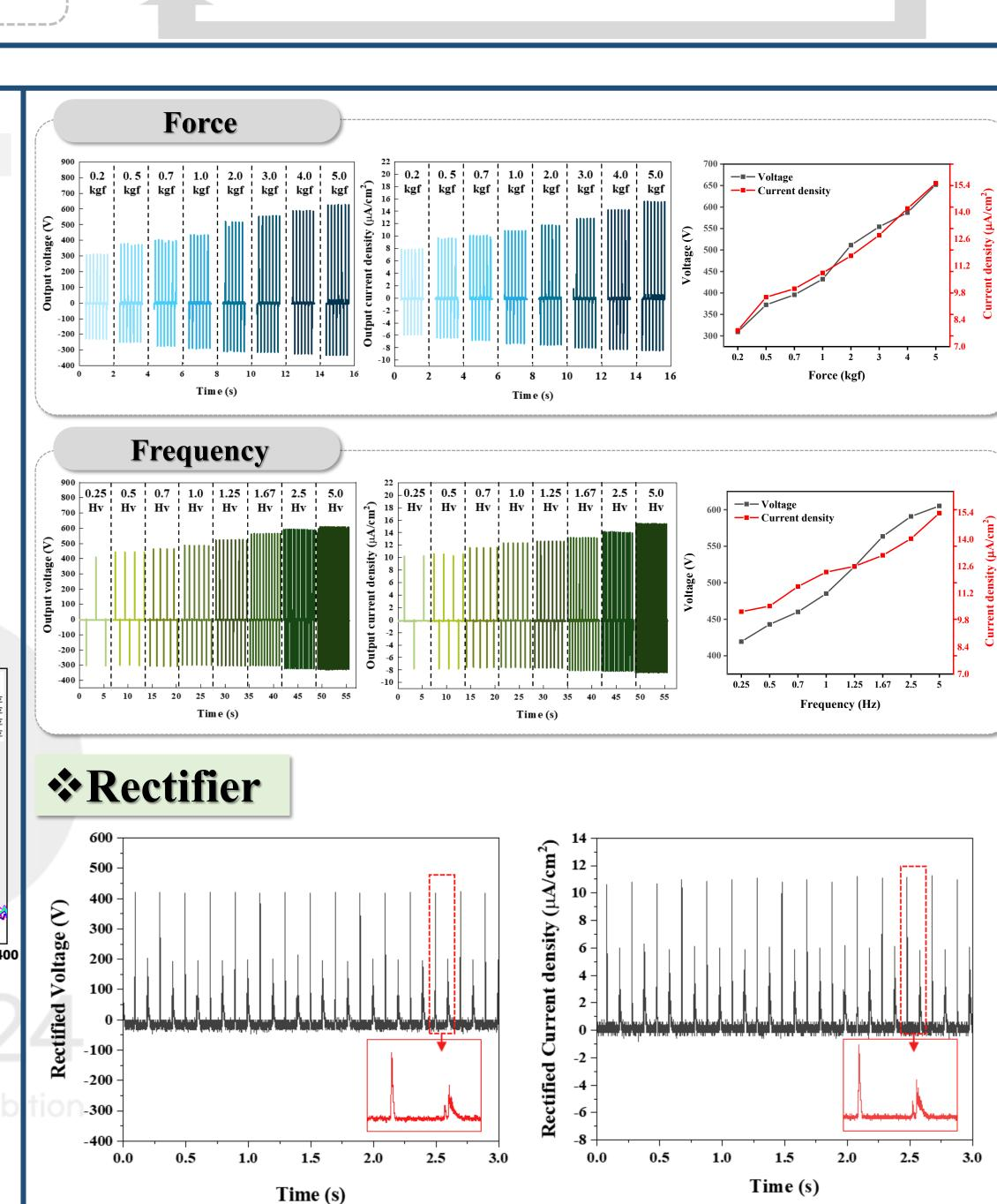
AC signals from the TENG were converted to DC using a bridge rectifier and stored in a capacitor
