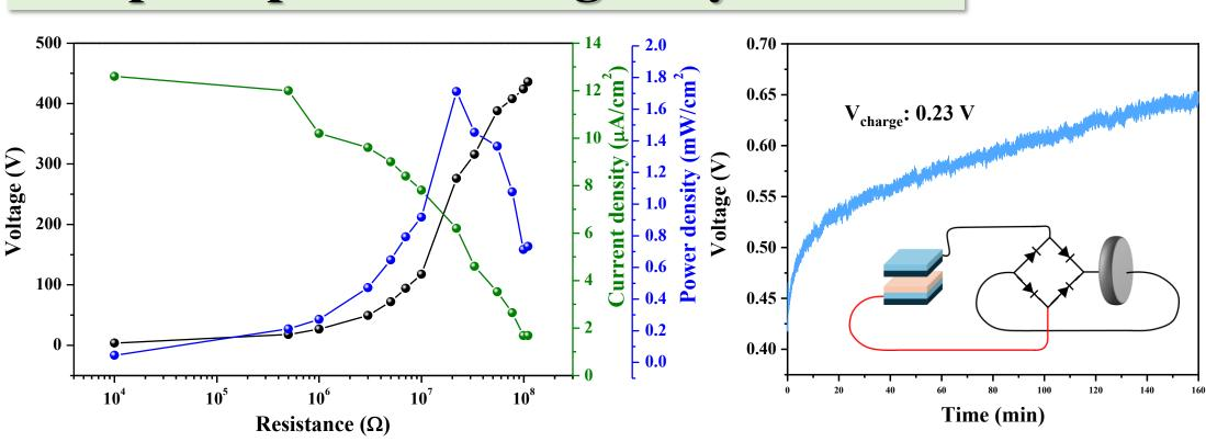
• Max. power density of 1.71 mW/cm<sup>2</sup> at matching load of 22 M $\Omega$
