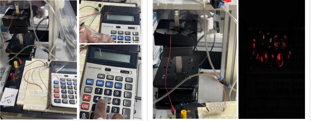
■ The TENG device powered a calculator and lit LEDs, showing its potential for daily-use self-powered applications
