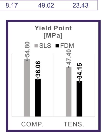
Compression and tensile tests were conducted on five specimens per process (SLS and recycled-PA12 FDM). The diagrams show:
