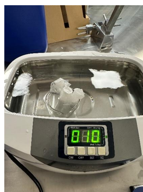
Figure 1. Paint mixtures on ultrasonic bath.
