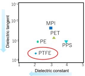
**Characteristics of PTFE** Low surface free energy Low maximum coefficient of friction Low dielectric constant and dielectric loss tangent
