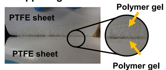
Other polymer gels peeled away from the interface, but this polymer peeled away from the middle.
