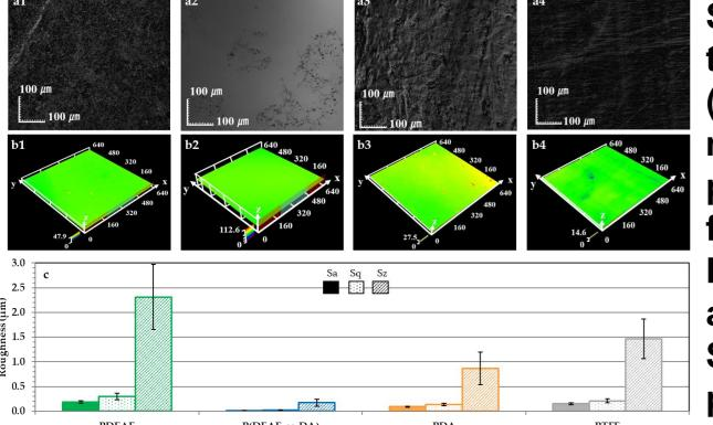
Surface characterization of three types of gels and PTFE. (a) Scanning mode digital microscopy images and (b) 3D profilometry reconstructions for (a1,b1) PDEAE, (a2,b2) P(DEAE-co-DA), (a3,b3) PDA, and (a4,b4) PTFE. (c) **Summary of 3D height** parameters (Sa, Sq, Sz).
