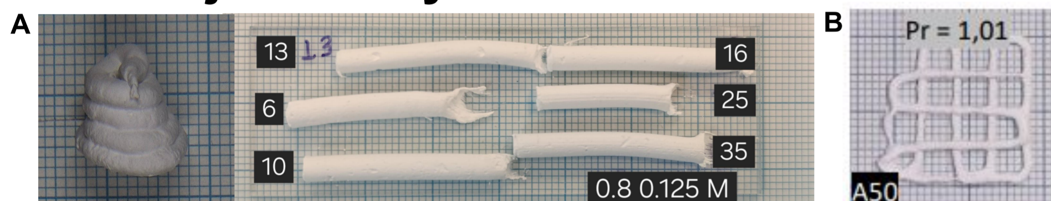
Figure 1: A. Smooth paste injection: representative images of the injected samples. B. Stable 3D printing: example of a well-defined, high-quality printed structure.
