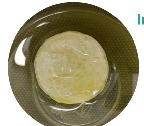
Impregnation of the aerogel in 30 mL of virgin fish oil at room temperature (±25°C). The sorption process was carried out passively until the aerogel reached saturation (1 hour).
