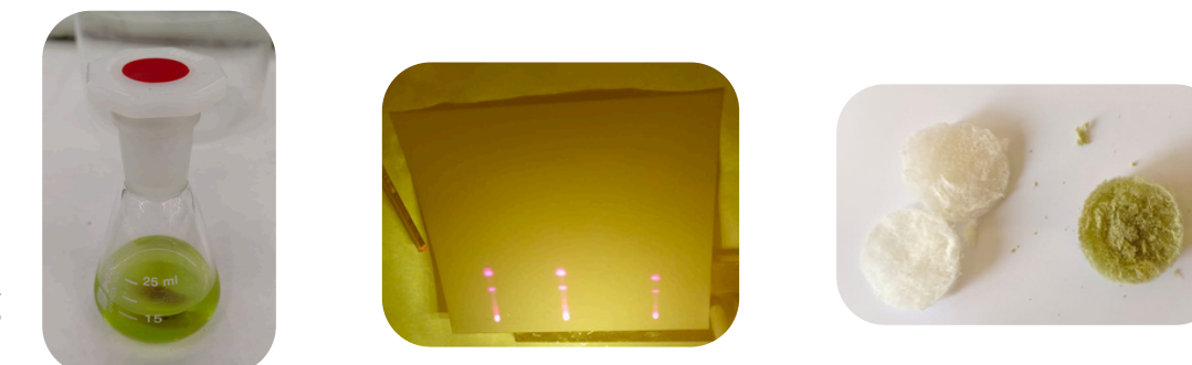
Figure 1. From left to right: a) Polyphenols extracted using the conventional method. b) Chromatogram of polyphenols. c) Agar extracted using the conventional method and assisted by ultrasound (green coloration).
