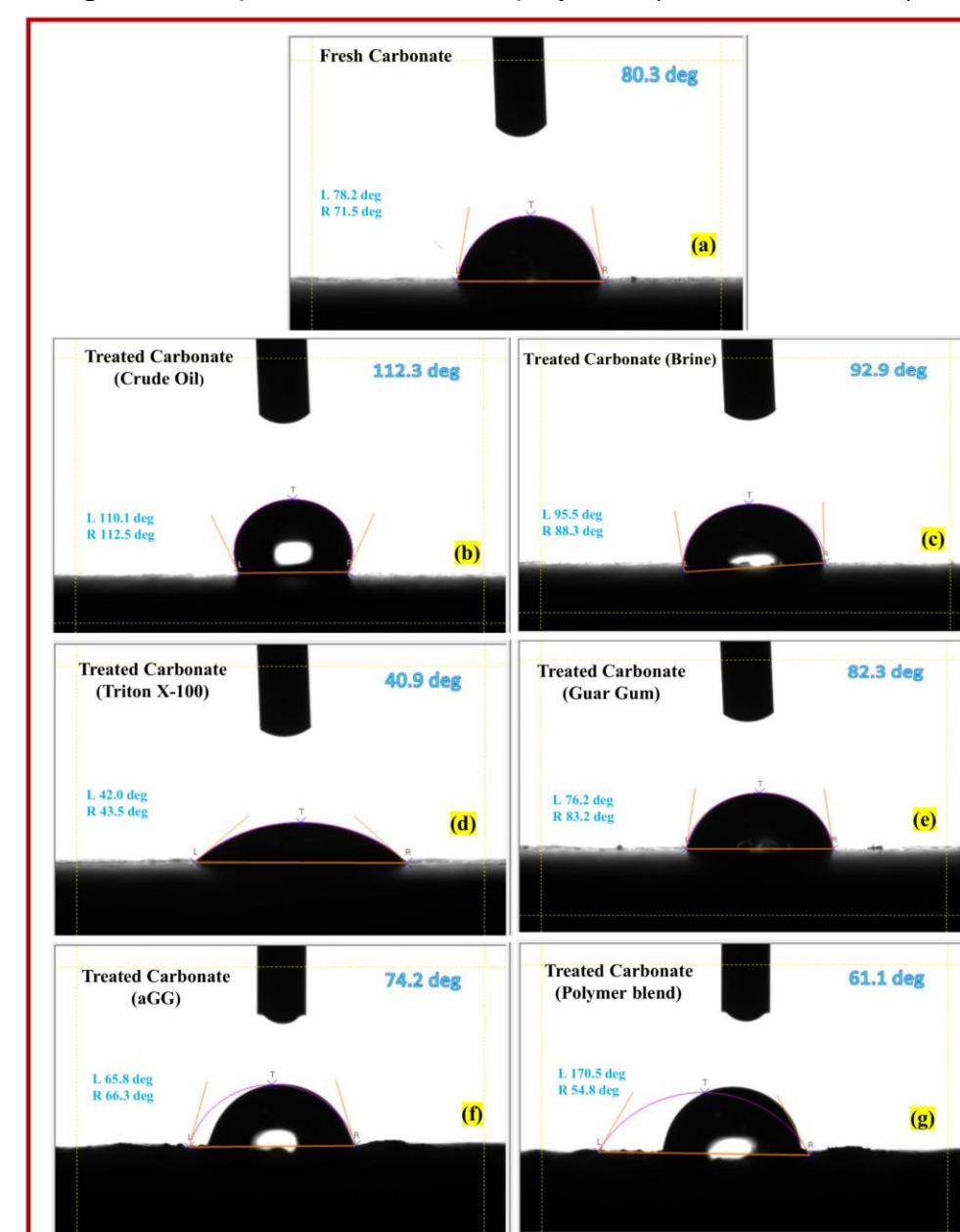
Fig. 11. Contact angle results showing enhanced wettability alteration, with the PB-treated carbonate surface exhibiting the greatest shift toward water-wet conditions
