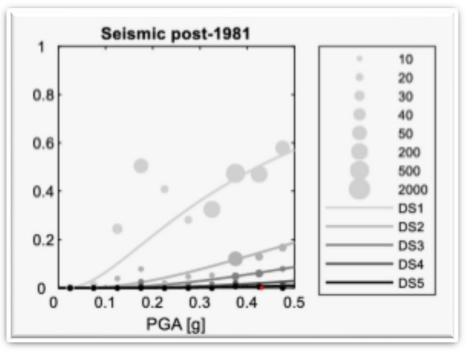
Fragility curves show how likely buildings are to sustain damage as earthquake intensity increases, supporting better mitigation and emergency planning. Rosti et al. developed widely used empirical fragility curves for buildings using Da.D.O. postearthquake data, fitting them with lognormal distributions to create national reference
