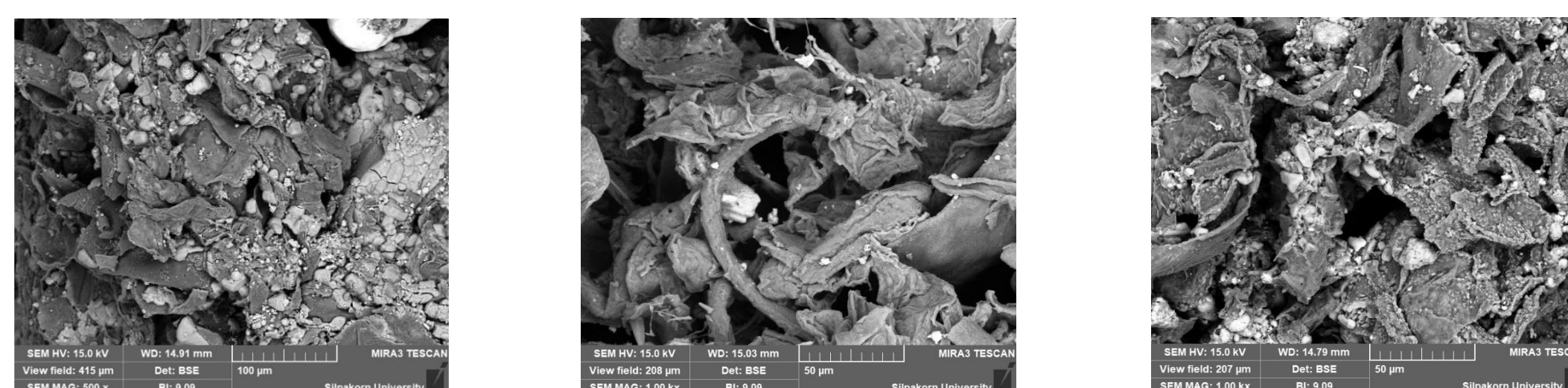
Fig. 1 SEM images of coated fertilizer with CMC at 2%, 5%, and 10% weight concentrations, captured at 500x magnification.
