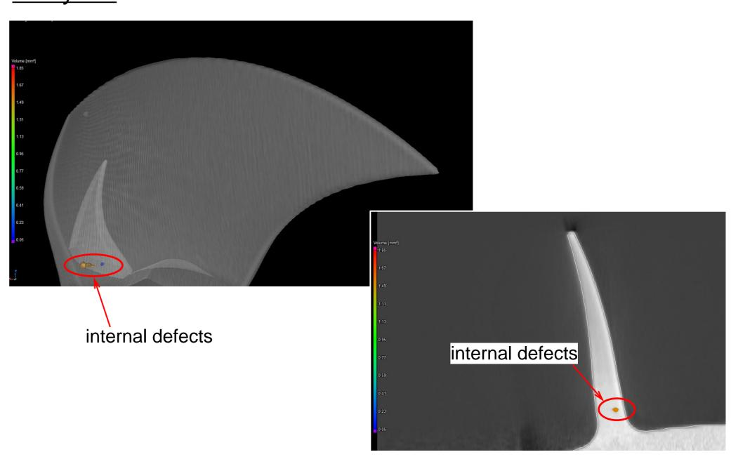
Several small internal defects detected
