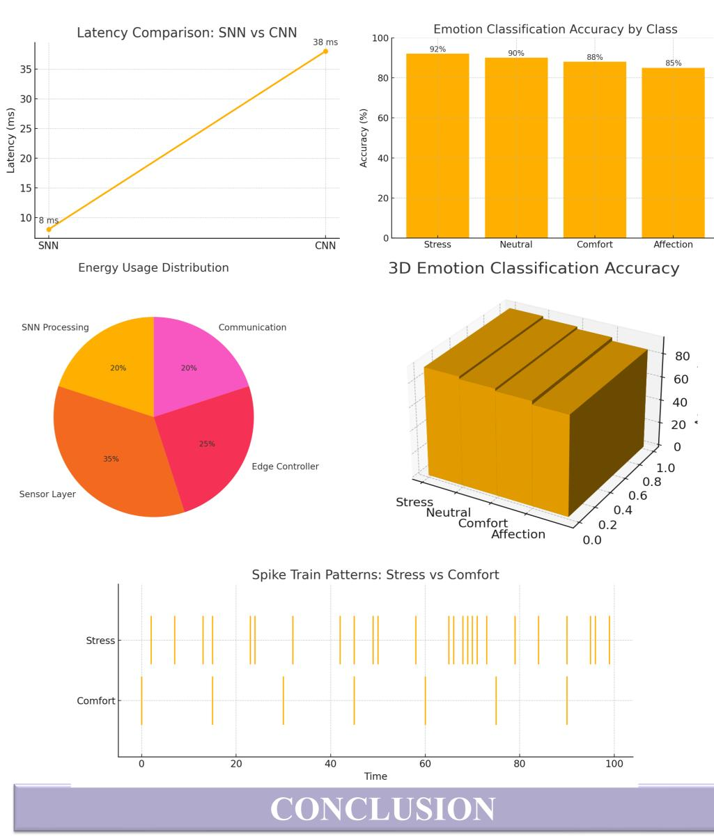
The neuromorphic multimodal e-skin effectively recognizes emotional touch with high accuracy and low latency. Its SNN-based processing significantly reduces energy consumption while maintaining real-time performance. Multimodal sensing enables clear separation of stress, comfort, affection, and neutral interactions. Overall, the system proves feasible for emotion-aware humanoid robots, enhancing safe and intuitive human—robot interaction.
