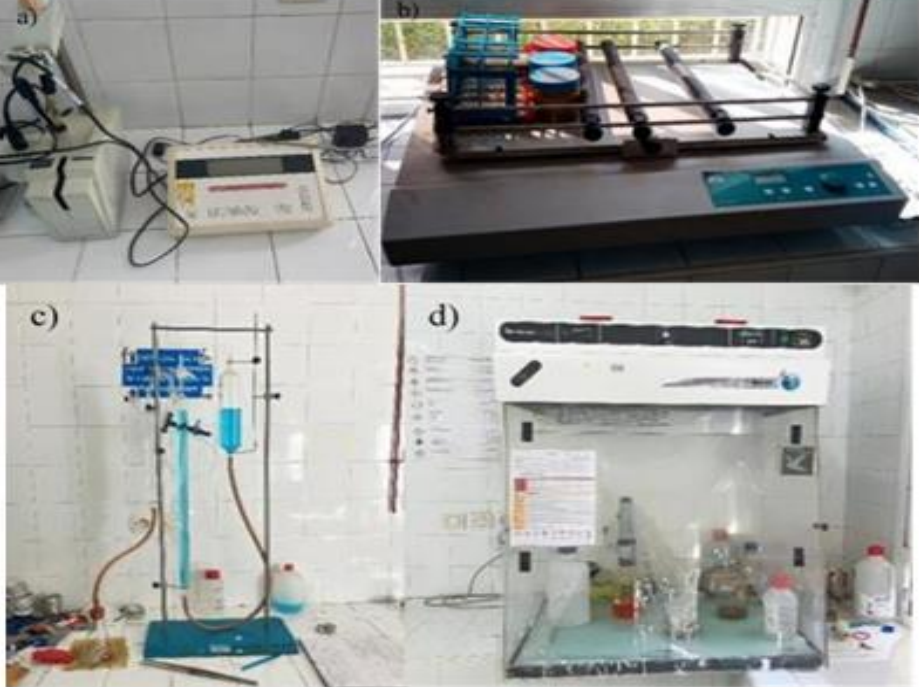
Figure 2. a. b) Materials used to measure pH, salinity, electrical conductivity, c) Calcium carbonate content, d) Organic matter
