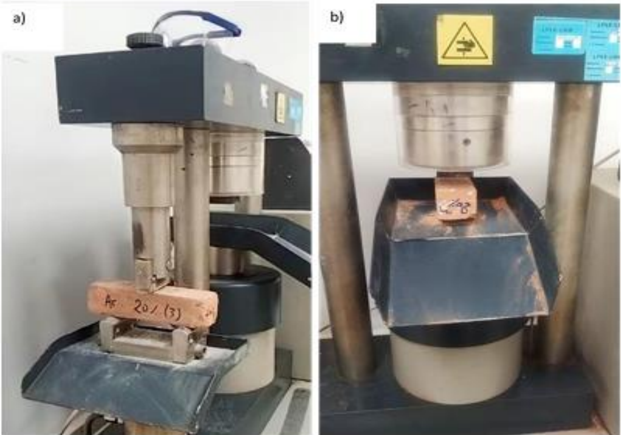
Figure 4. Mechanical test on (4x4x16 cm3) prisms of adobe bricks
