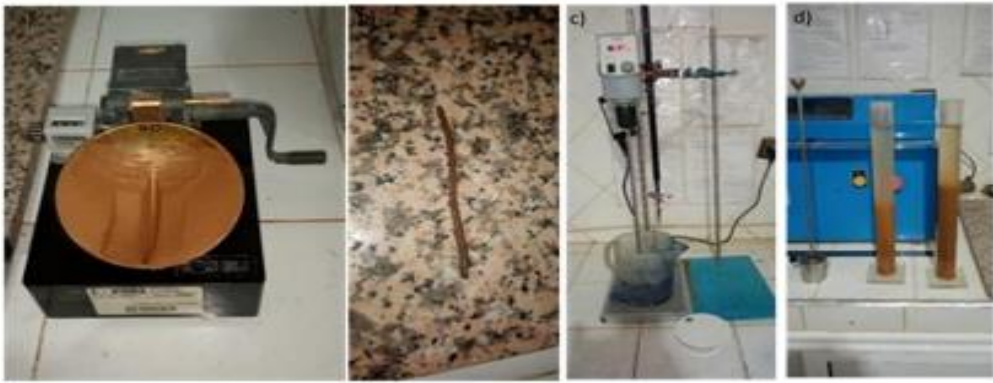
Figure 1. Techniques used to measure geotechnical soil properties: a. b) Atterberg limits, c) Methylene blue, d) Sand equivalent
