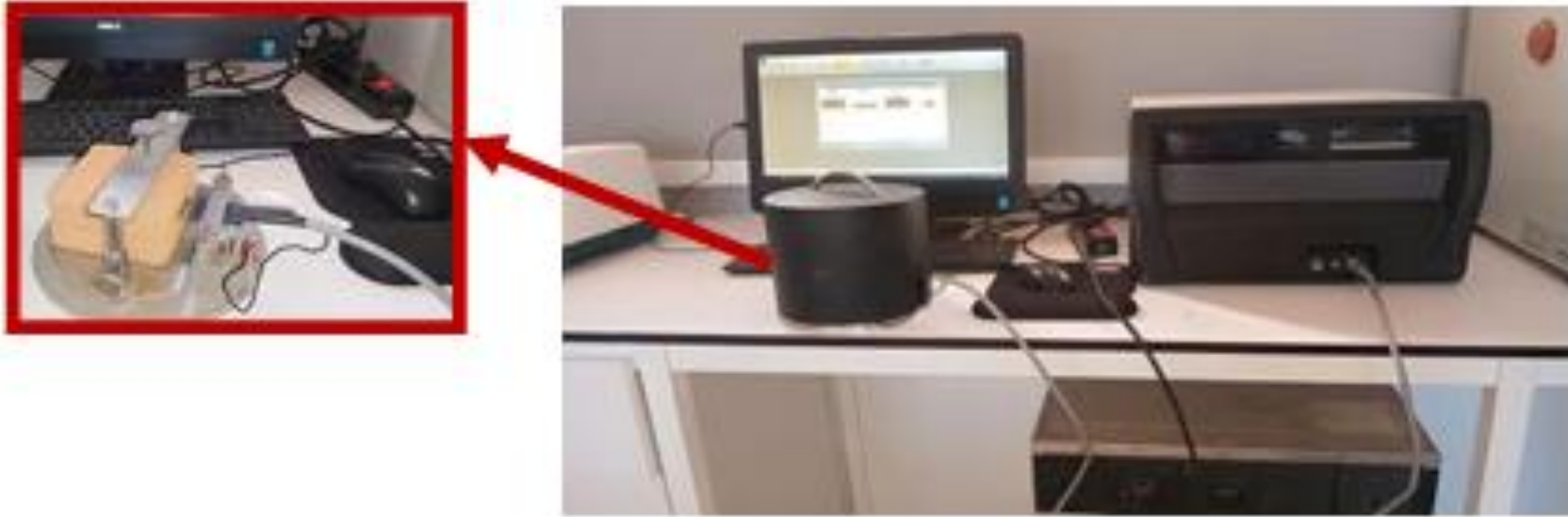
Figure 3. Thermal test on (10x10x2,5 cm3) prisms of adobe bricks
