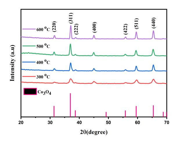
JCPDS Card No: 01 - 074 - 1656Crystal Structure: Spinel Cubic phase Space Group: Fd3m
