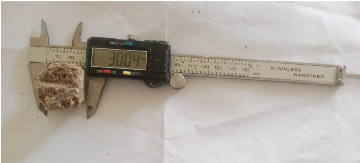
Fig 4: Determination of the mould efficiency using Vernier caliper
