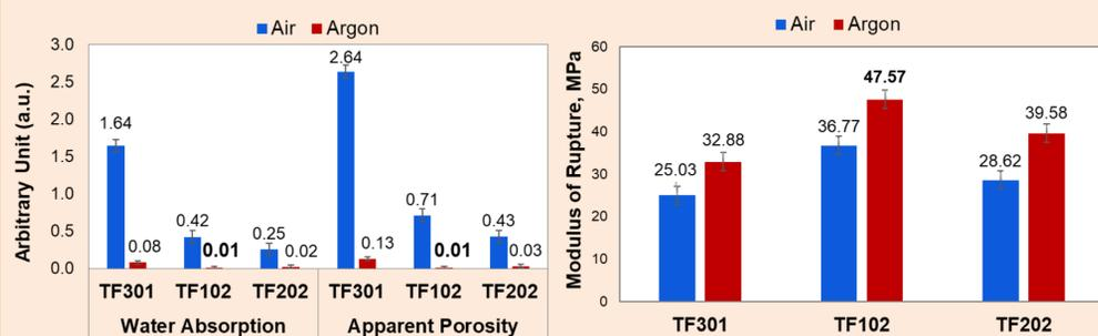
Figure 1. Water absorption, apparent porosity and modulus of rupture (MOR) of red clay-black cinder ceramic bodies sintered under air or argon atmosphere.
