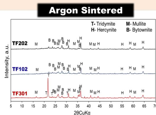
Figure 2. XRD patterns and corresponding SEM micrographs of red clay–black cinder ceramic bodies: (a) TF301, (b) TF102, and (c) TF202, sintered at 1200 °C under an argon atmosphere.
