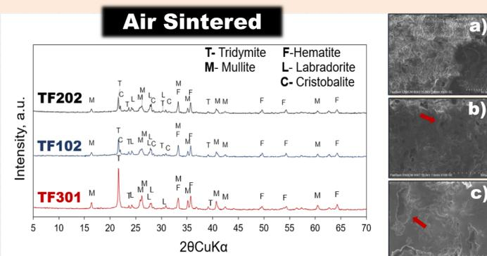
Figure 2. XRD patterns and corresponding SEM micrographs of red clay–black cinder ceramic bodies: (a) TF301, (b) TF102, and (c) TF202, sintered at 1200 °C under an air atmosphere.
