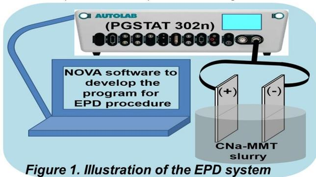
Figure 1. Illustration of the EPD system
