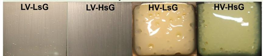
Figure 4. Wet Na-MMT deposits after EPD
