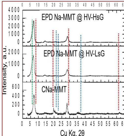
Figure 5. XRD of Na-MMT powders after EPD
