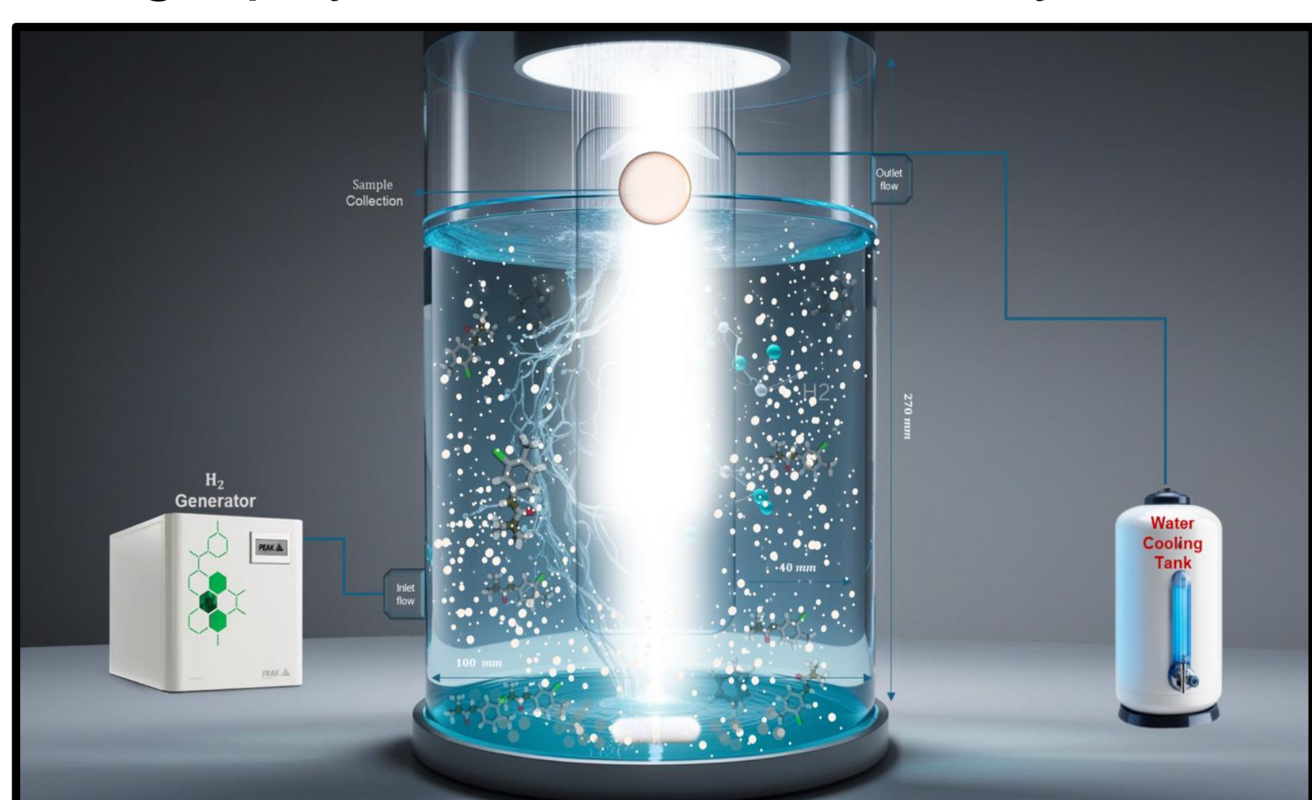
Fig. 1. Schematic diagram of UV reactor, connected with H 2 generator connected with rotameter to regulate flow and water cooling system.
