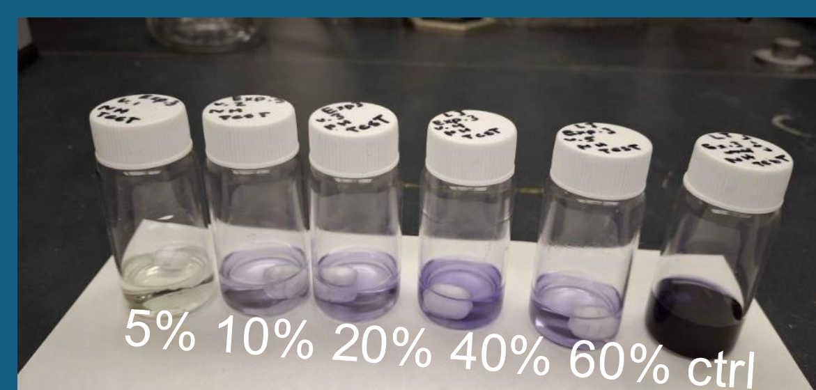
Figure 2: Results of Ninhydrin test showing a deeper color correlates to more APTES present on silica
