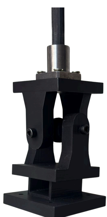
Fig. 4. 3D Printed Universal Joint with Flange bearing
