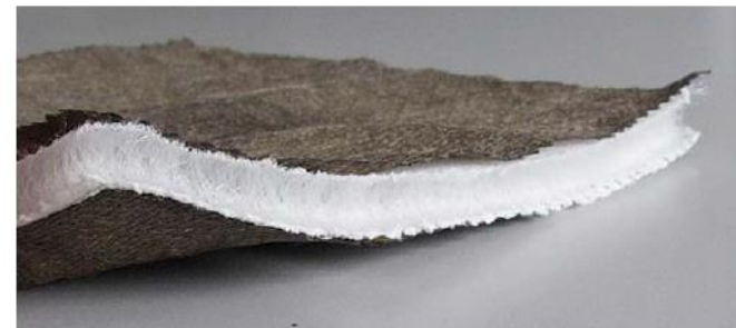
Capacitive textile sensor
