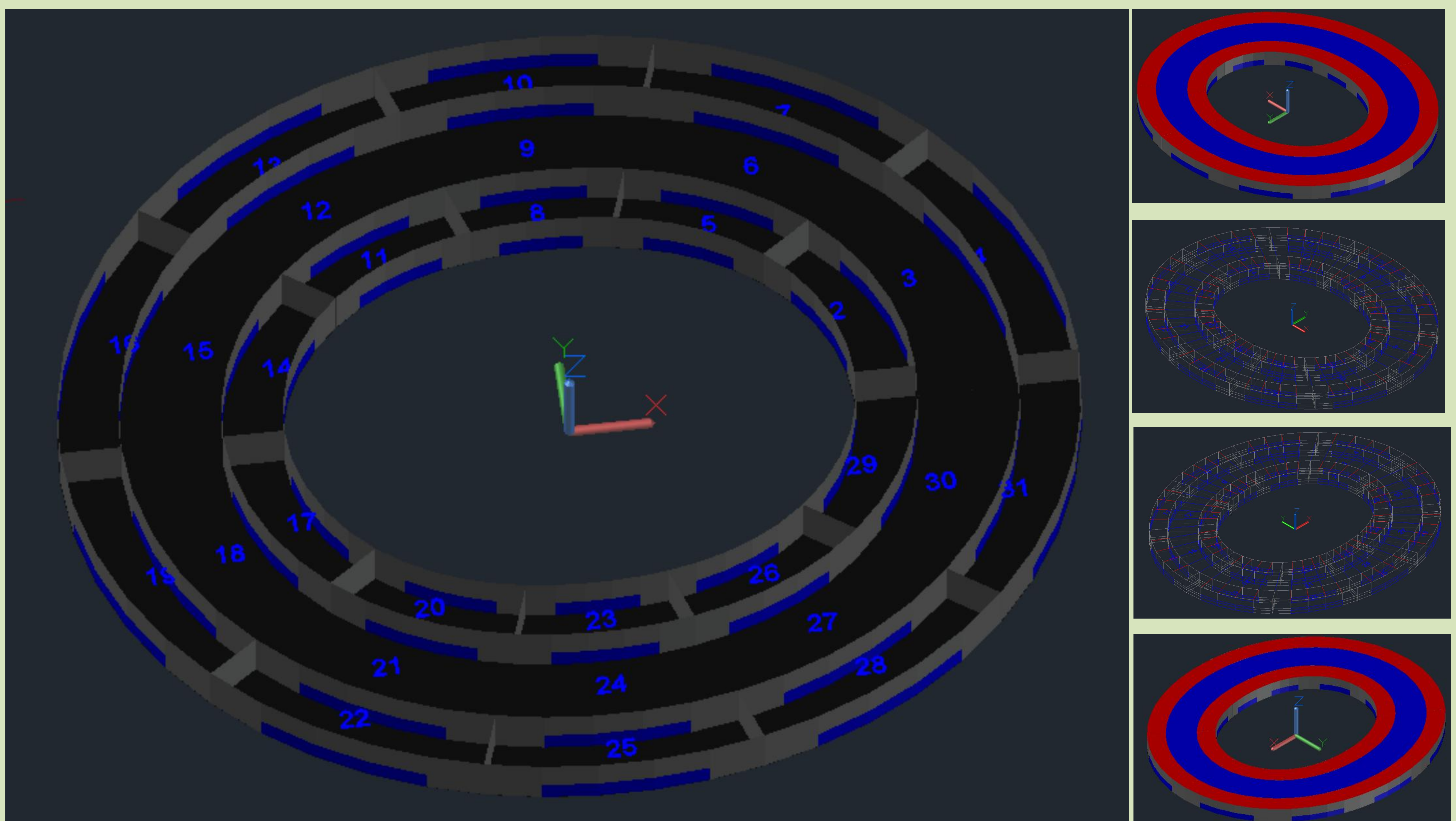
Figure. Opaque bodies (grey), as internal and external bodies, transparent bodies (blue) as windows and doors, and roofs (red).
