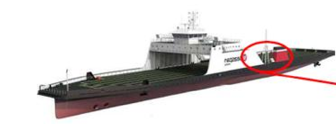
Location of Bunkering manifold for both LIN and LNG filling:
