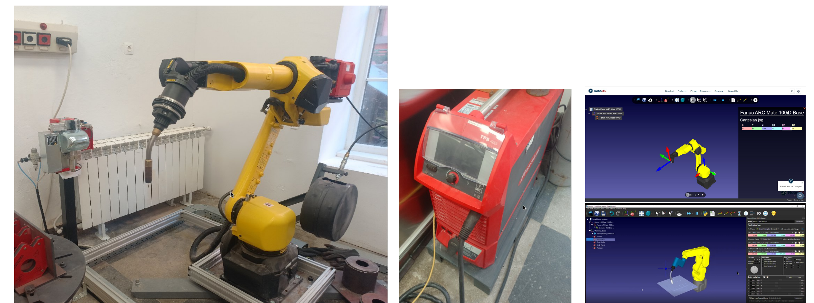
Figure 3 DED-arc application setup with software simulation
